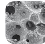
The unique production process leads to porous ceramics, resembling the structure of human cancellous bone with fully interconnected pores.
