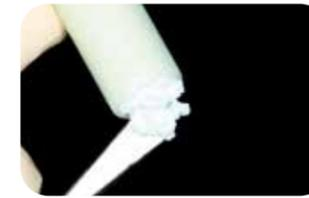
The maxresorb® inject paste is brought to instrument for application
