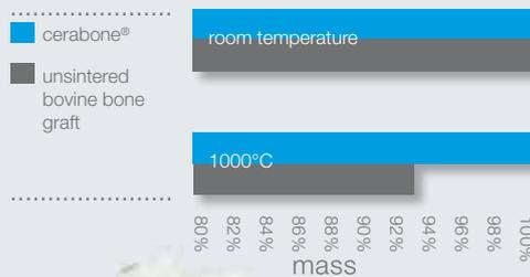
Thermogravimetric analysis showing combustion of organic components.
